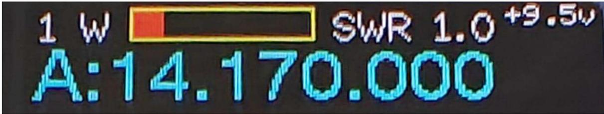
Figure 10 - Power and SWR meter
