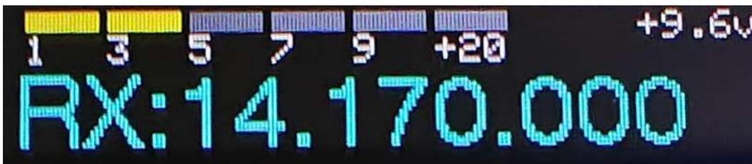
Figure 11 - VFO with RIT enabled
