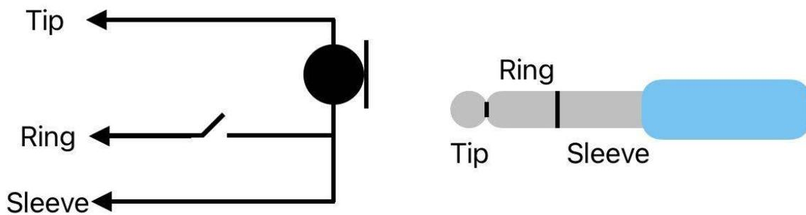
Figure 19 - PTT microphone wiring
