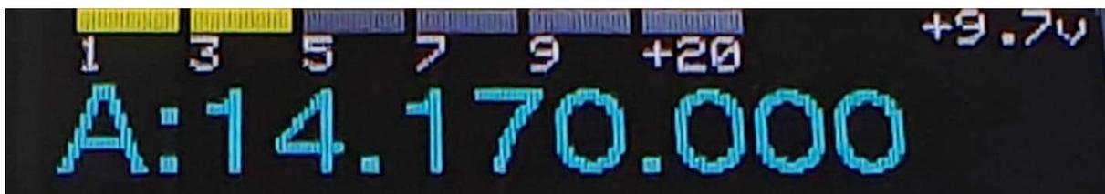
Figure 09 - VFO, S-Meter & Battery Voltage Monitor
