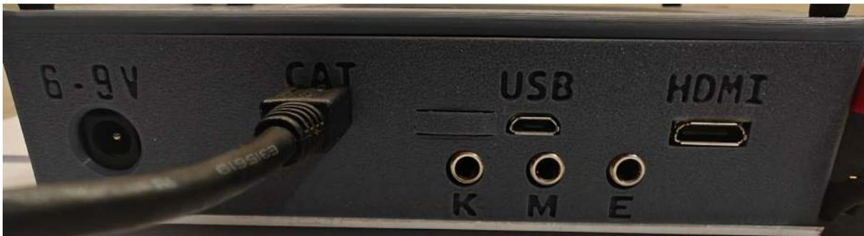
Figure 21 - USB Cable connected to CAT connector
