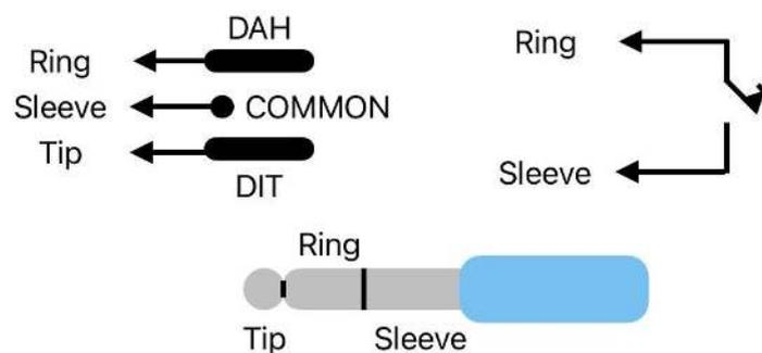
Figure 14 - Paddle/Key wiring
